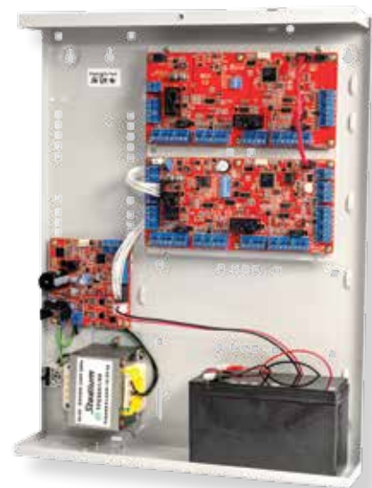
ABOVE: ILAM shown in 4 Door / 4 Reader configuration. (ILAM with UniBus 2 Door / 2 Reader expansion device connected) Housed in the Medium size 995201PEI enclosure with 3Amp Power Supply.
